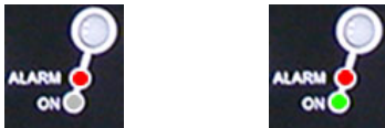
Port Error (unable to power on) Port Error (unable to power off)
