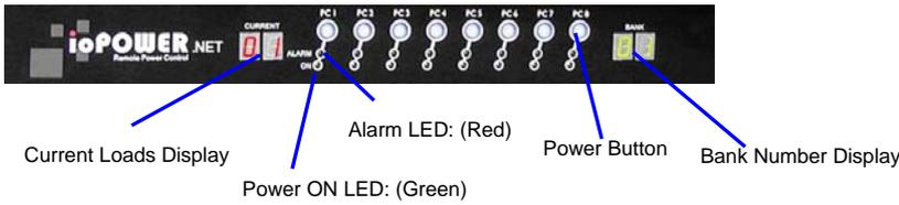
To actuate an outlet by using the front panel, press and hold the corresponding button for over **two seconds**. The port is toggled upon button release.
